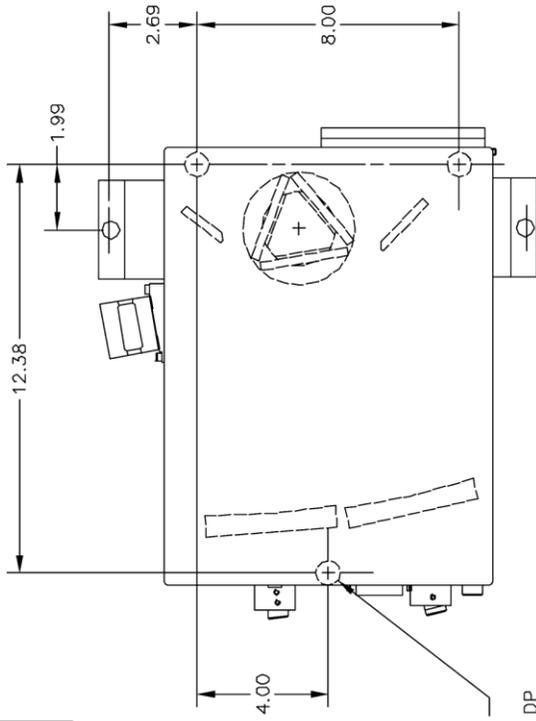
LOCATION OF THREE (3) SUPPORT PADS ON THE BOTTOM SURFACE WITH #8-32 TAPPED HOLES, 3/8 DP
