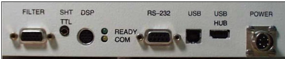
Figure 10. Cable Connections (Back Panel)
