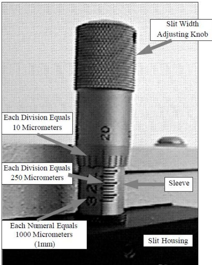
**Figure 7. Slit Width Setting:
