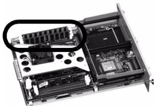
2. Push out the white lock tabs at either end of the DIMM socket.
