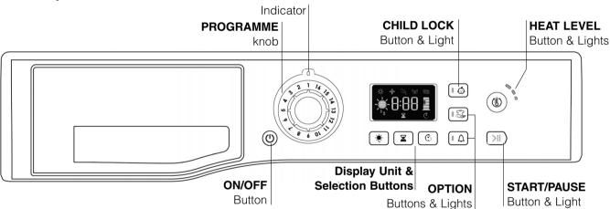
The **ON/OFF** button (1): If the drver is running and this button is pressed and held for more that 3 seconds the dryer is turned off, it counts down 3, 2, 1, Off and the programme is then cancelled.
