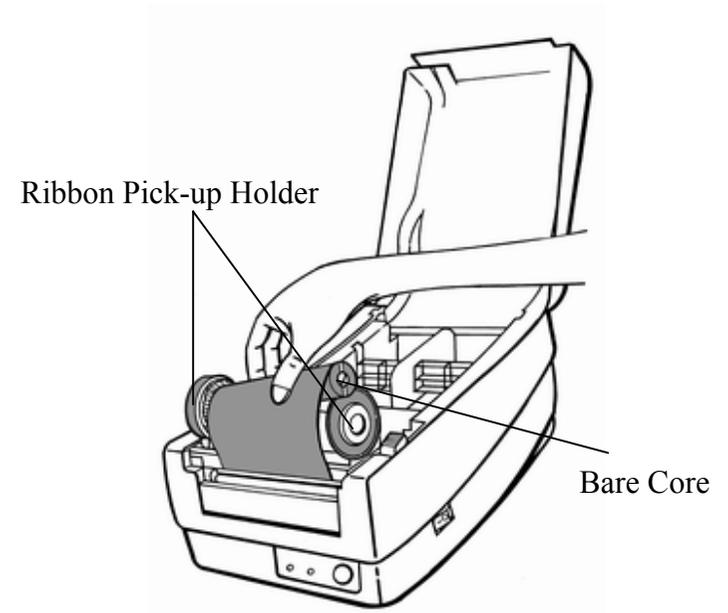
8. Turn the wheel of the print head module to ensure the ribbon is tightly wound.
