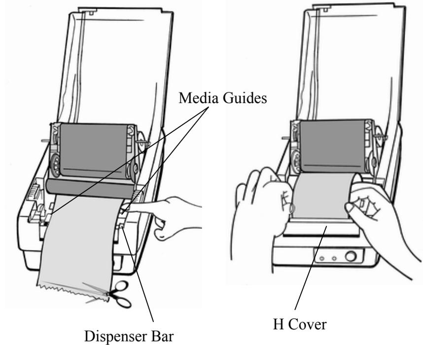
12. Press "FEED" button and the label backing paper will come out from the slot under the H cover.
