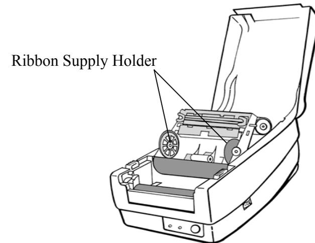
4. Unwrap the ribbon roll pack and separate the ribbon roll and the bare core.
