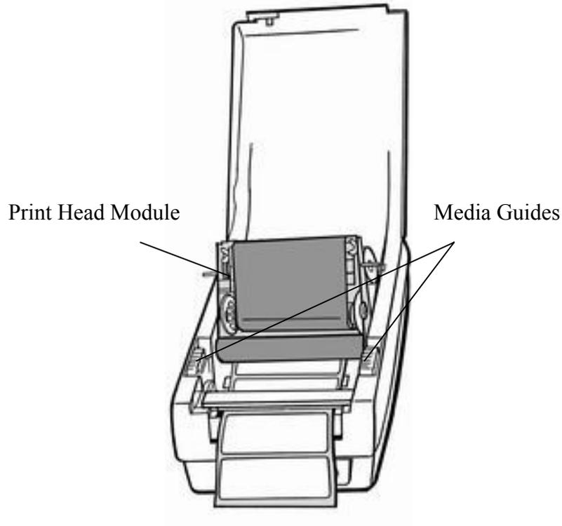
10. Turn back the print head module and then press it down firmly till you hear a snap.
