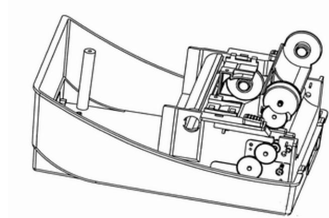
13. Unlatch the print head module. Hook the white roller on the brackets of the chassis, ensuring the long thinner end at the left side.
