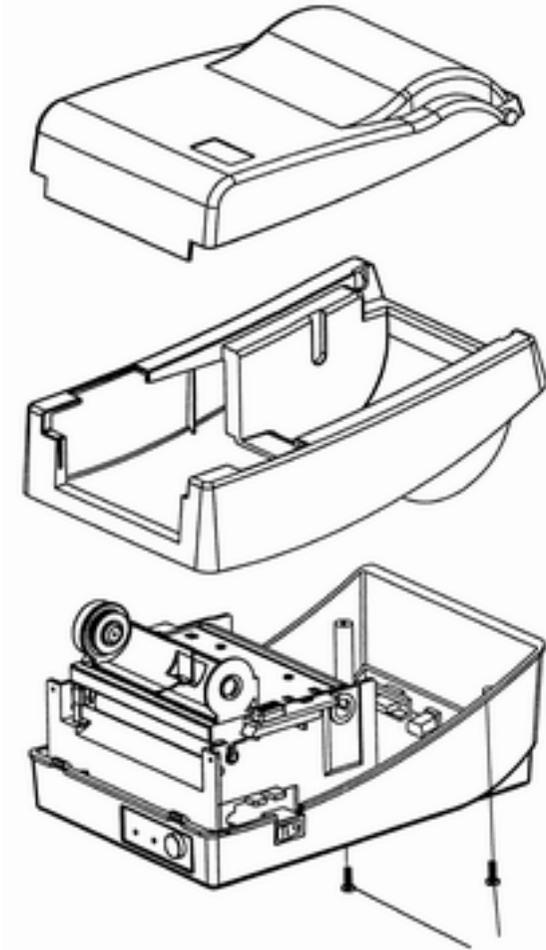
4. Remove the whole print head assembly by releasing 4 screws at its feet.
