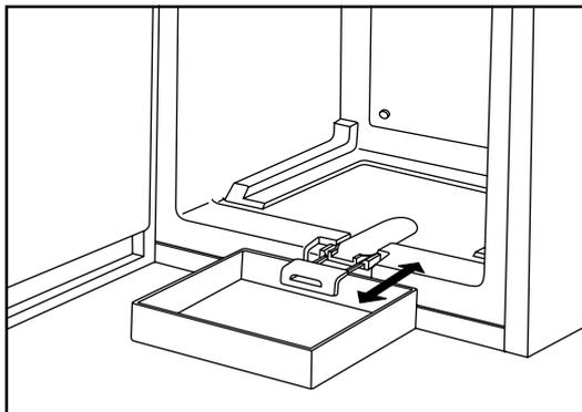
5. During defrosting, push the defrost water towards the edge of the cooling plates using a dry cloth or a sponge. It will be collected at the bottom of the appliance, from where it can be diverted into the tray and then disposed of.
