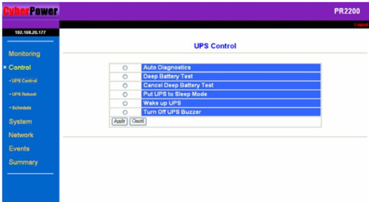
[UPS Control] allows basic remote control of the UPS.
