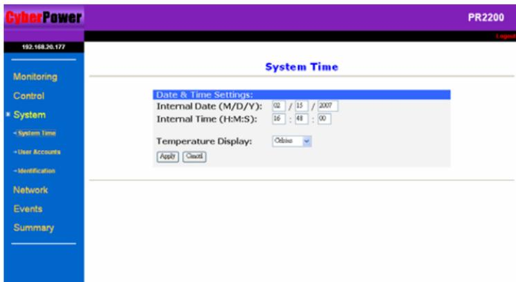
[System Time] allows users to configure the internal time of the Network Management Card .
