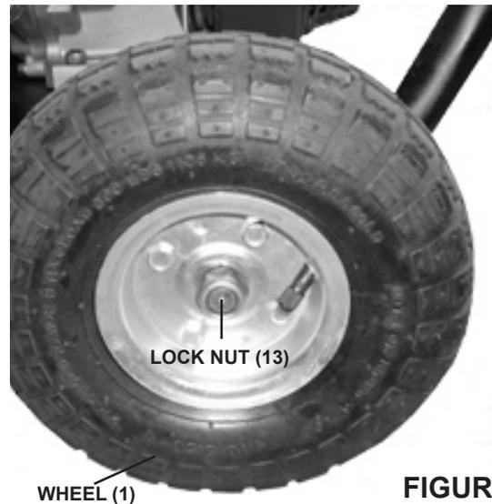
3. To attach the Wheels (1), slide a Wheel onto each end of the Axle located at the front of the Frame (2). Make sure air valve on wheel faces outward. Then secure the Wheels to the Axle, using one Lock Nut (13) for each Wheel. (See Figure B.)
