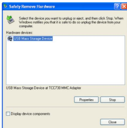
When the message “Safely Remove Hardware?” is displayed, click the <OK> button and then unplug the USB cable from the product.
