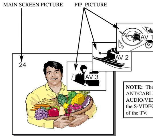
**NOTE:** The PIP source picture can come from the ANT/CABLE input, the AUDIO/VIDEO AV1, the AUDIO/VIDEO AV2, the AUDIO/VIDEO AV3, or the S-VIDEO input jacks located at the rear and side of the TV.
