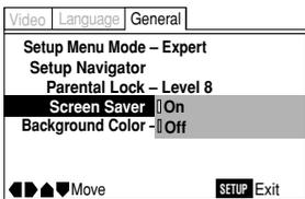
If a constant image is displayed on a conventional CRT-type TV, it can “burn in” leaving a ghost image on the screen. When **On**, the screen saver makes sure that a constant image is not displayed for a dangerously long time.
