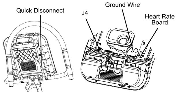
(c) With the display electrical connections made, you can now attach the display. There are 2 tabs located on the bottom of the display weldment, so in order to attach the display, you will first need to guide the bottom of the display under the tabs and then second you will need pivot the display forward around the tabs to mate the display to the rear plastics. Once in place, you can attach the screws.
