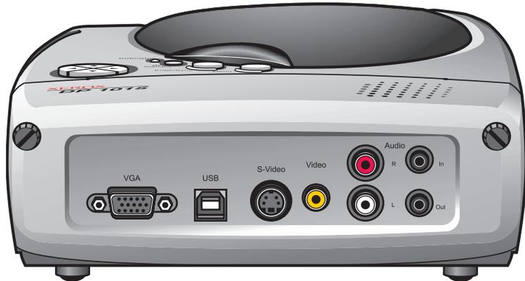
**VGA Port**—Plug the VGA cable into this VGA port, and plug the other end into the video port on your computer. Use this port to project video from your computer with the projector.
