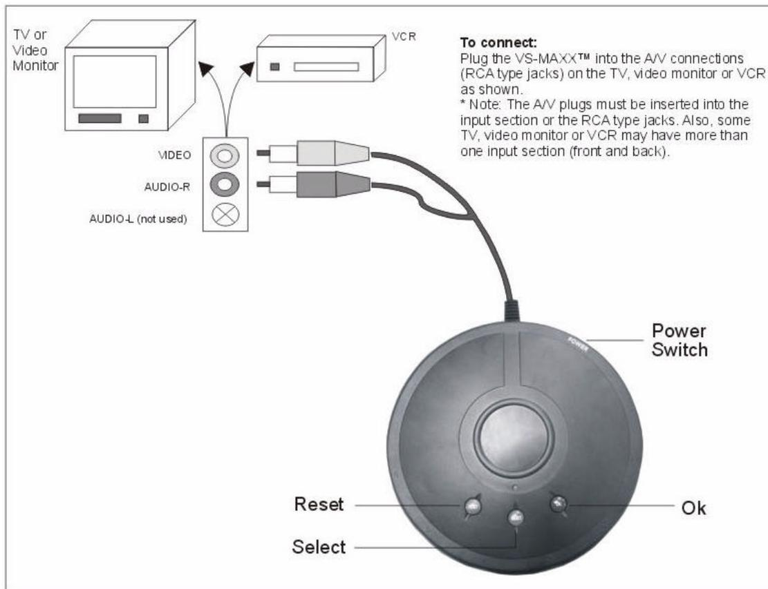
*Note: The A/V connections will be located either in the front or back of your TV, video monitor or VCR. The A/V plugs must be connected to the standard "input" RCA type jacks. The plugs are color coordinated to the "input" jacks (red-audio and yellow-video). If your TV, video monitor or VCR does not include standard "input" RCA type jacks, you will need to purchase a separate A/V adaptor (not included).*
