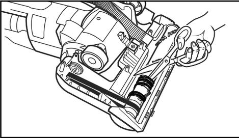
➤ Remove any string or debris located on the end caps, washers or agitator shaft.
