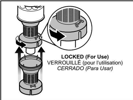
➤ **Rotate pre-filter clockwise to lock in place.**
