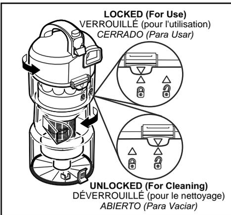
➤ **Reinstall dust bin lid and turn to locked position (as indicated on the lid).**
