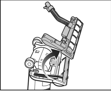
➤ Clean agitator after every five uses and every time the belt is replaced.
