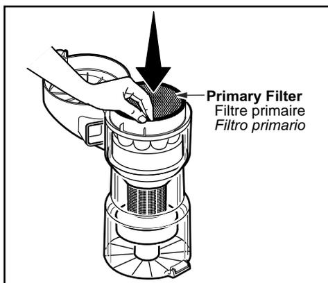
It is recommended to clean the filter with cold water at least every three (3) months. Check the primary filter frequently and clean when dirty.
