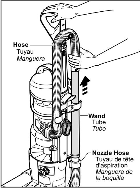
**NOTE:** Hold the handle to support the vacuum cleaner when using tools and disconnecting or attaching the hose.
