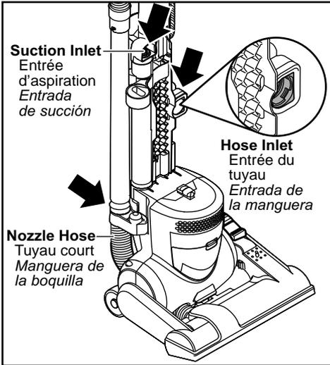
If the vacuum cleaner does not seem to have adequate suction, first check if the dust bin is full or if a filter is clogged.
