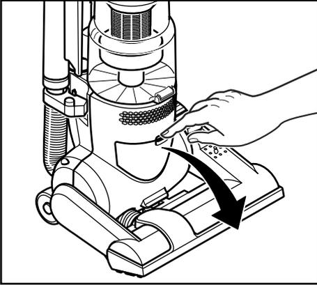
The HEPA media exhaust filter removes dirt from exhaust air. Check filter after emptying dust bin. Replace when dirty.
