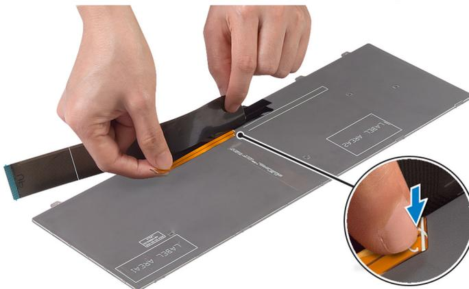
3. Using the alignment line, fold the keyboard cable.
