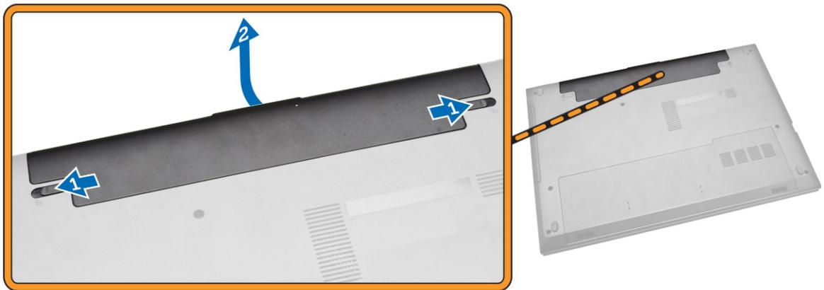
3. Lift the battery to remove it from the computer.
