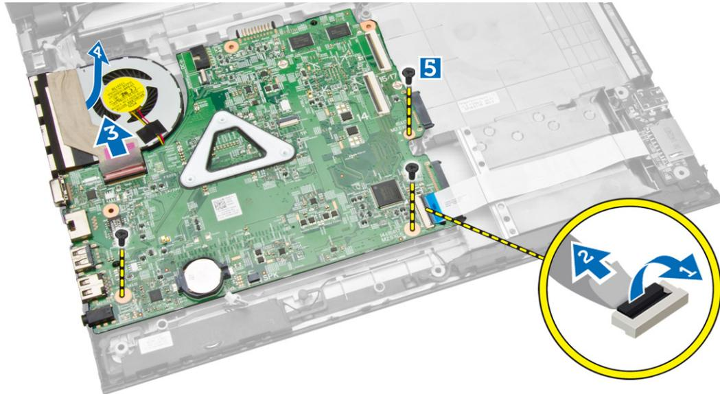
5. Lift and remove the system board from the chassis.
