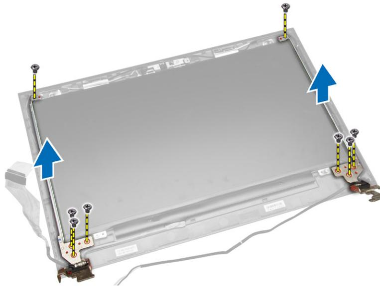
6. Remove the screws securing the display panel to the display assembly. Then, flip the display panel to access the cables underneath.
