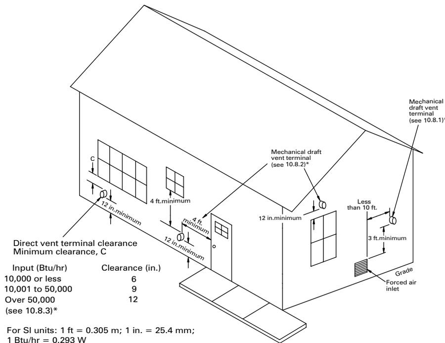
EXIT TERMINALS OF MECHANICAL DRAFT AND DIRECT-VENT VENTING SYSTEM
