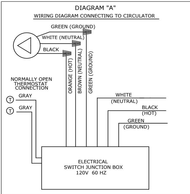
Figure 2-1: Connection Wiring Directly to Central Heating Circulator
