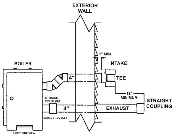
**\*\*IMPORTANT NOTE:** All vent pipes must be glued, properly supported and the exhaust must be pitched a minimum of a 1/4" per foot back to the heater (to allow drainage of condensate).
