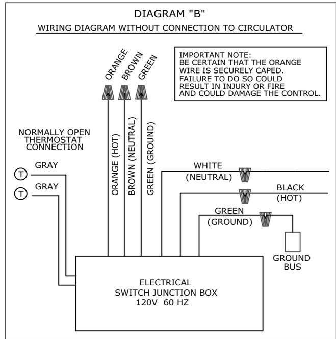
Figure 2-2: Connection Wiring without Wiring Central Heating Circulator
