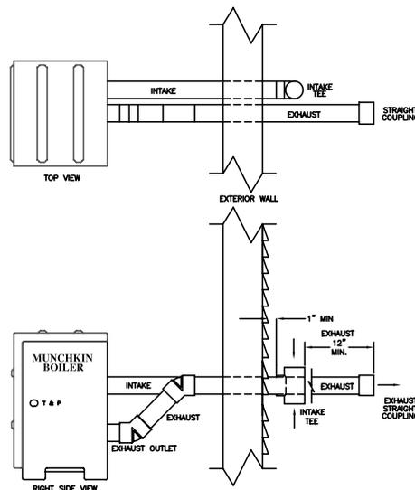
**SIDEWALL VENT WITH TEE (INTAKE) & COUPLING (EXHAUST)
