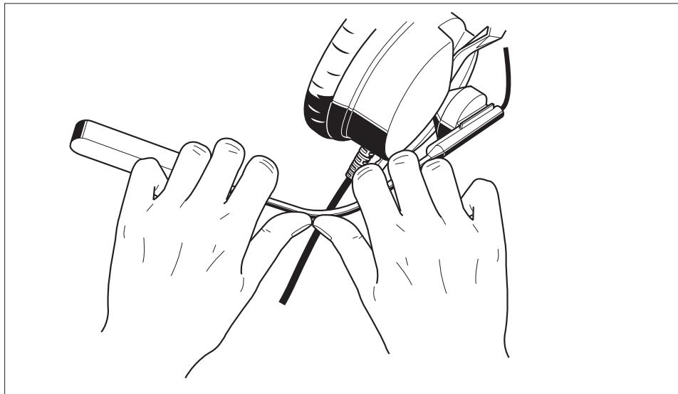
**N.B.:** The microphone boom is adjusted for an individual user. However, care should be taken when doing this. Once set, the boom should not be re-adjusted. If it is continually flexed it is liable to break.
