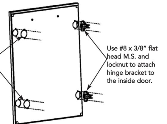
7. Cabinet doors must be adjusted when cabinets are level in final position. There are two adjustment screws on the hinge receiver. (See Illustration #5)
