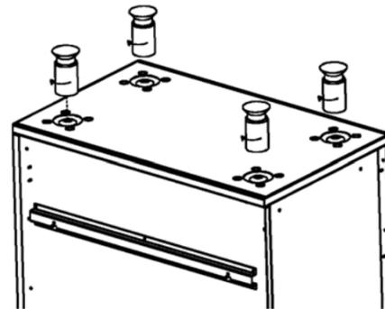
5. Place cabinet(s) in approximate final position. Level cabinets using leveling legs. Use 1/2" SMS screws provided to screw cabinets together. (See illustration #3).
