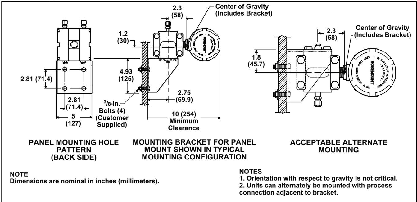
Figure 2-5. Transmitter Dimensional Drawings.
