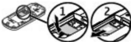
Press the release spring (1), and slide out the SIM card (2).
