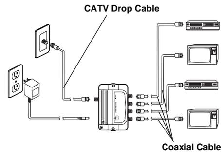
**Caution:** Use only coaxial cable (not supplied) to make the connections. Your local RadioShack store carries suitable cable.
