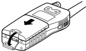
3. Insert three (3) AA ALKALINE batteries according to the polarity symbols on the inside of the battery compartment.
