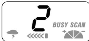
3. To exit from this weather channel mode, press the **wx/ctcss** button again.
