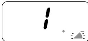
When the batteries in the unit are low, the unit will go into a Battery Low/Sleep Mode. The Scan Mode, Monitor Mode, Transmit, Transmit Call Tone Mode, CTCSS Tone Setting Mode, VOX Sensitivity Level Setting Mode, and Vibration are disabled. Replace the batteries immediately to continue using the radio.
