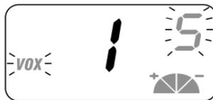
4. Within 10 seconds, select one of the level numbers, 1 (the lowest sensitivity) ~ 9 (the highest), using the **up** or **down** button.
