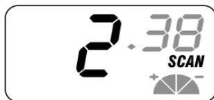
If a signal is present, the radio will stop on the active channel. It will remain on the channel until the transmission ends. After 2 seconds, it will resume scanning.
