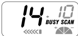
2. To resume scanning prior to the transmission end, press **scan/vibrate** again.
