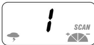
2. Scanning stops when the radio finds an active channel. It stays on the channel until its transmission ends, and resumes scanning after a 2 second delay.
