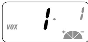
3. To set the VOX sensitivity level, press the **call/vox** and **scan/vibrate** buttons simultaneously until the VOX icon and number indicator begin to flash.
