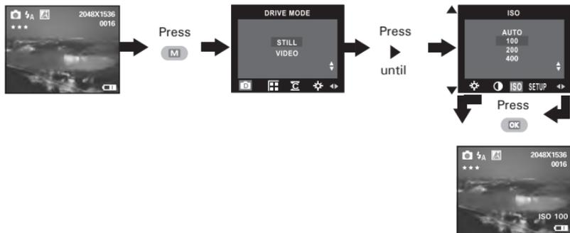
**AUTO** The camera's sensitivity is automatically detected by different lighting value or subject brightness.
