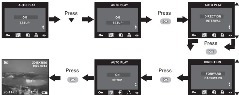
Press the up or down button to choose the direction in which the camera will automatically run, and then press the OK button to confirm your choice.
