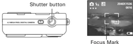
5. Press the Shutter button completely down to take a picture while holding the camera steady. A beep will sound (if the Beep sound is turned on) when a picture is taken.
