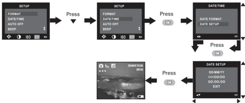
Use the ◀ or ▶ button to select a field, such as year, month, day, hour, minute. Use the ▲ or ▼ button to adjust the value in the field. Press the OK button after all fields are set.
