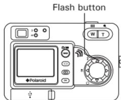
When you press the Flash button, the icon (according to the flash setting you selected) will appear on the LCD screen. You can now take pictures using the flash mode you selected. The flash will recharge after each flashed picture.
