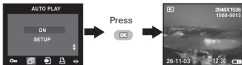
The camera will automatically run from the first file or from the last file stored. Every file will display for the specified period according to your interval setting. You can press the left or right button to manually skip backward or forward. You may press the OK button to pause or press the Wide Zoom button to stop the auto play. The auto play will keep running as long as there is power.
