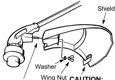
**NOTE:** Remove and use washer and wing nut from this bolt for assembling shield.
