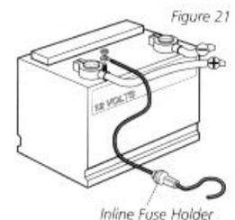
The Power can be connected to the boat's electrical system at two places: a fuse panel, usually located near the console, or directly to the battery.
