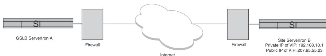
Using the example in [Figure 3](#), suppose the configuration specifies that the public IP address will be used by both the peer GSLB ServerIron ADX A and the site ServerIron ADX B. If ServerIron ADX B is providing GSLB in addition to being a site ServerIron ADX, and has a local site configured, then it will also use this public IP address of the VIP for its local site.
