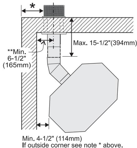
For corner installation, Restrictor must be set at 1-1/4" open.
