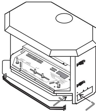
To adjust the aeration: use the allen key to turn the turning gear which will adjust the air shutter. Open the air shutter for a blue flame or close it for a yellow flame. The factory setting should be sufficient for most installations.
