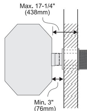
For straight rear installation, Restrictor must be set at 1-1/8" open.
