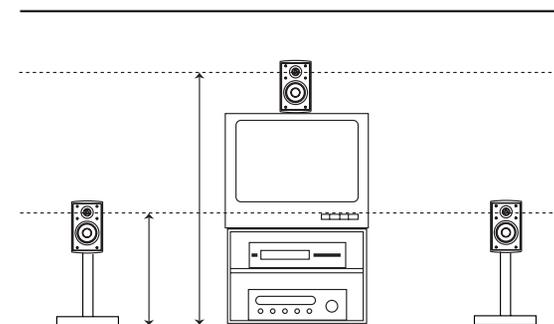
**Figure 3** Improper placement of left/center/right front speakers.
