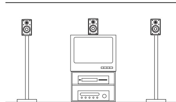
**Figure 2** Proper placement of left/center/right front speakers.
