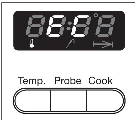
When using the "Cook" button or the roasting probe, the residual heat of the oven is automatically used to finish the cooking process and conserve energy.
