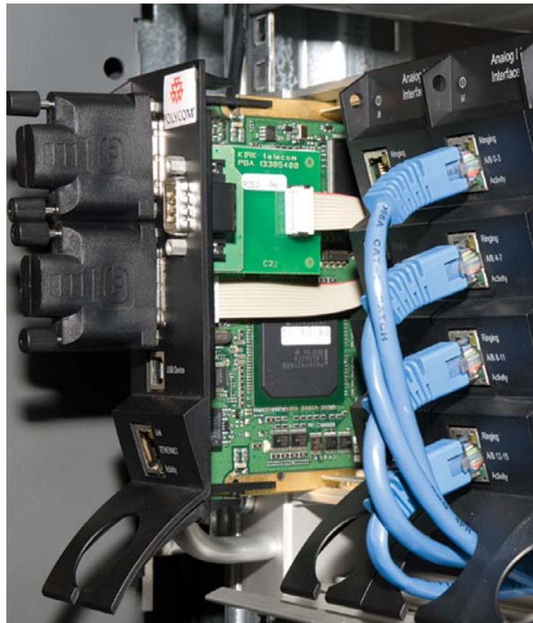
Figure 1-7 Installing CPU card
