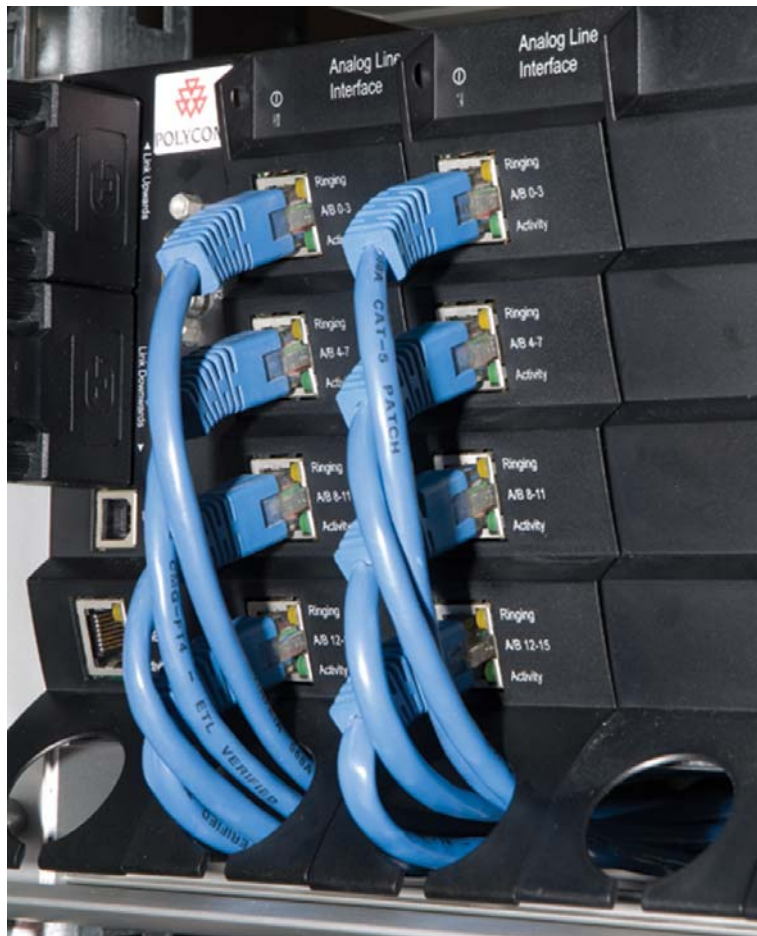
Figure 1-8 Harnessing cables to the back and out
