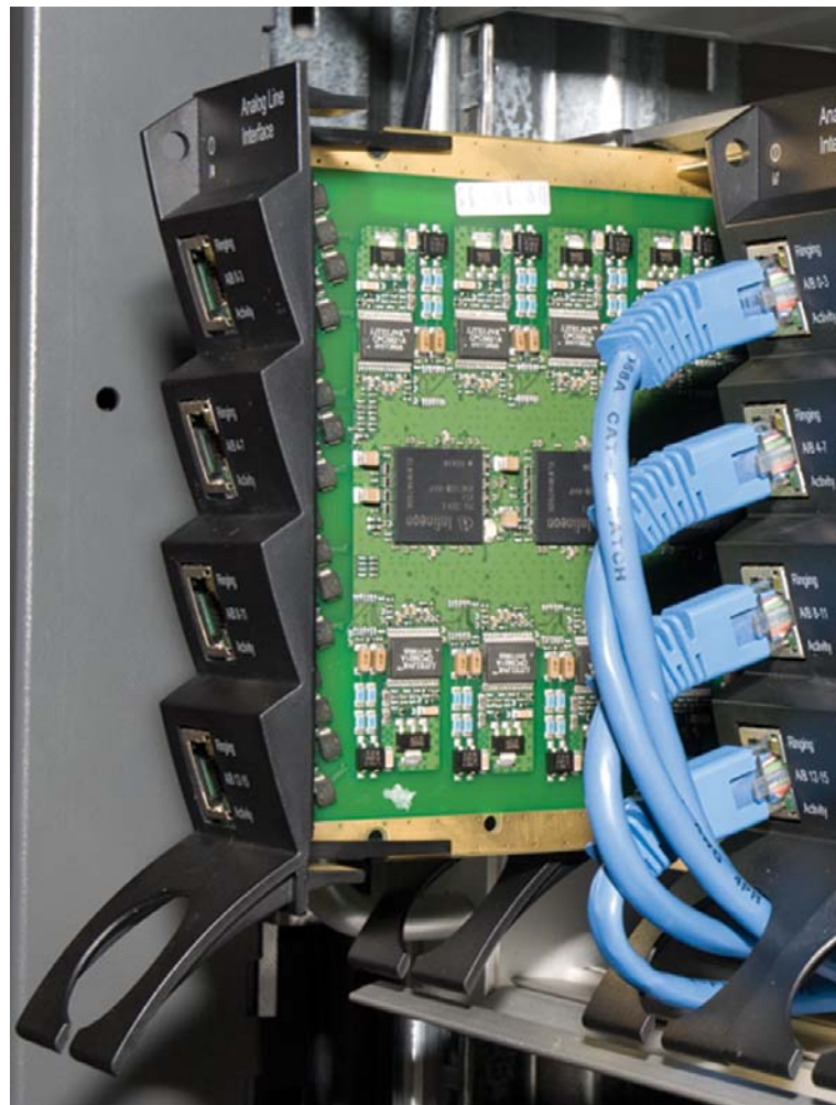
Figure 1-6 Installing Interface cards
