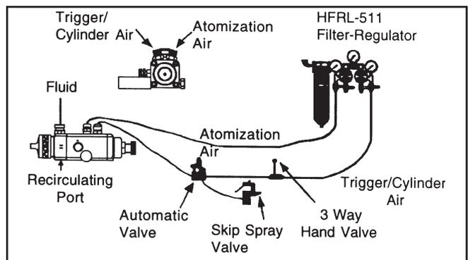
Attach the trigger/cylinder air hose and the atomization air hose to the connections as indicated by the markings on the gun body. The air supply should be filtered and regulated. Attach the material hose to the fluid inlet on the gun body. Fluid can be recirculated by installing a fluid fitting (AGX-415) (order separately) at the recirculating port. See **Caution** below.
