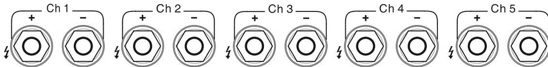
Each – and + speaker terminal will accept bare speaker wire up to AWG 12, a wire terminated with a ¼" spade lug, or with a single banana plug; dual banana plugs which are ¾" (19mm) apart may be used for each speaker.
