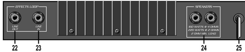
**22. EFFECTS LOOP LINE OUT:** When using an external effects processor, connect this jack to the input of the effect by means of a shielded signal cable. This jack also doubles as a source for a post-EQ, preamp signal to send your signal to a mixing board, recorder, powered monitor or external amplifier.
