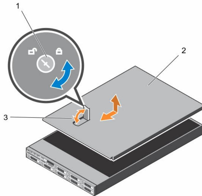
**Figure 15. Removing and installing the system**
