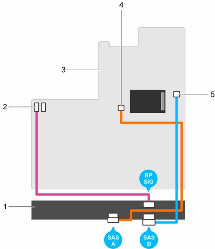
**Figure 49. Cabling diagram—2.5 Inch (x8) systems**
