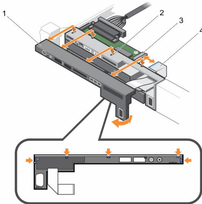
**Figure 55. Removing and installing the control panel**
