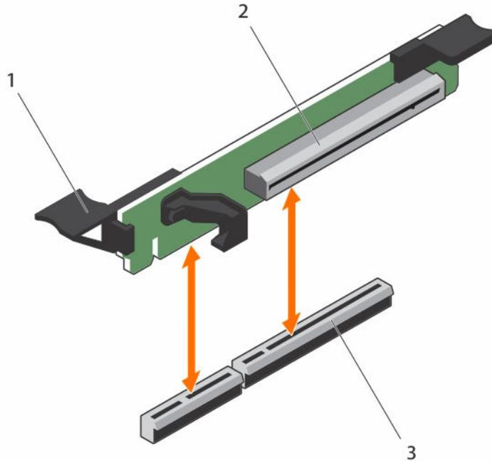
**Figure 34. Removing and installing the expansion card riser 3**
