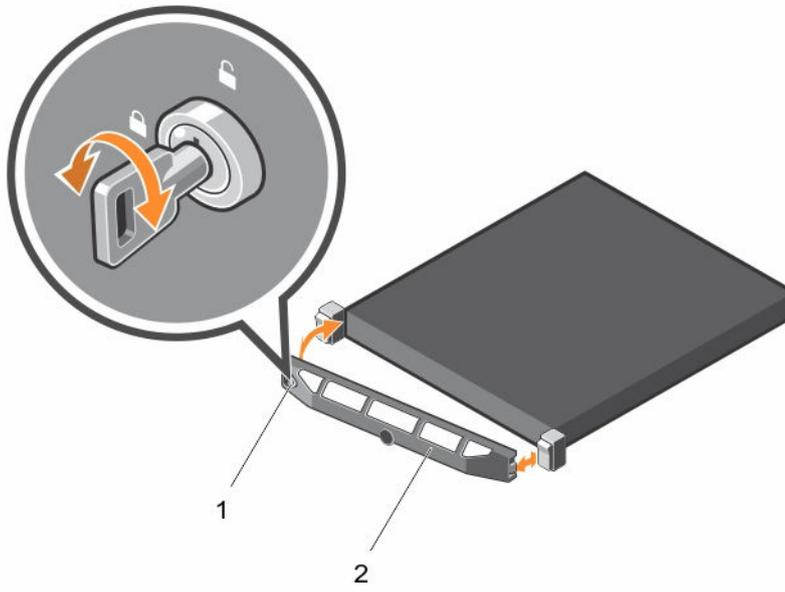
**Figure 13. Removing and installing the front bezel**
