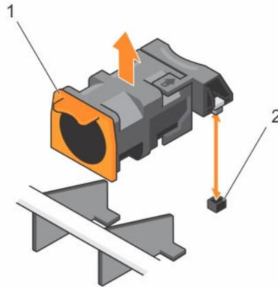
**Figure 30. Removing and installing a cooling fan**
