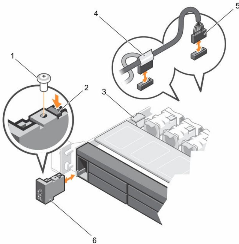
**Figure 56. Removing and installing the control panel**
