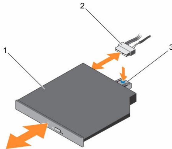
**Figure 28. Removing and installing the optical drive**
