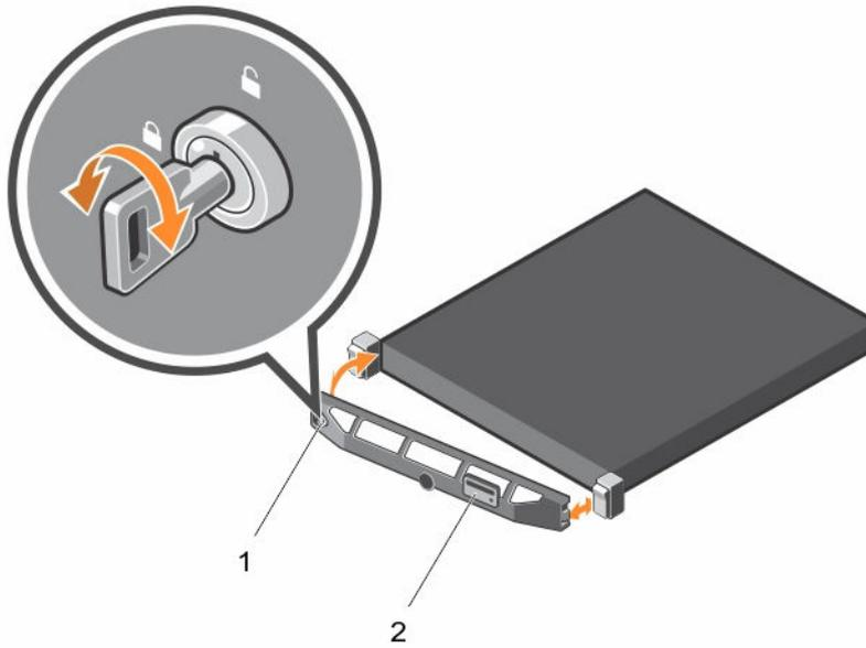
**Figure 14. Removing and installing the Quick Sync bezel**
