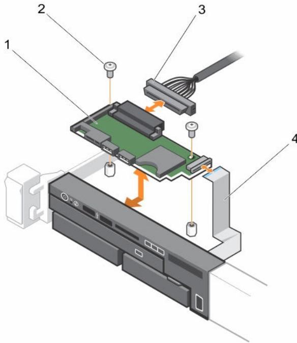
**Figure 54. Removing and installing the control panel board**
