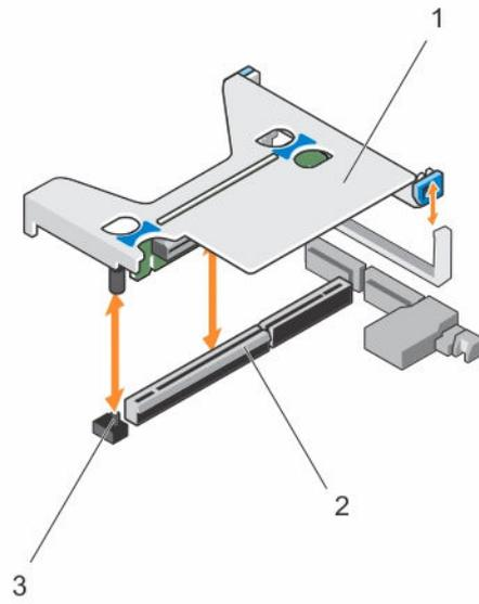
**Figure 33. Removing and installing the expansion card riser 1**
