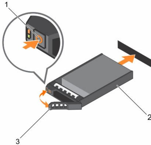
**Figure 24. Removing and installing a hot-swappable hard drive/SSD**
