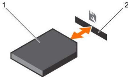
**Figure 35. Removing and installing the SD vFlash card**
