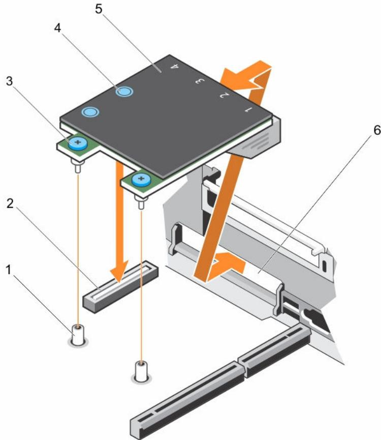
**Figure 38. Removing and installing the network daughter card**
