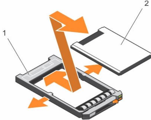
Figure 27. Removing and installing a 1.8 hard drive into a hard-drive carrier
