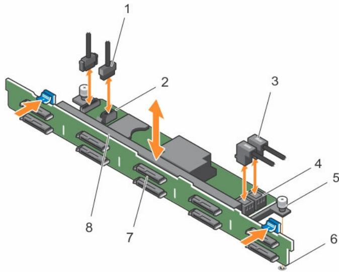
**Figure 50. Removing and installing the 2.5 Inch (x10) hard-drive backplane**
