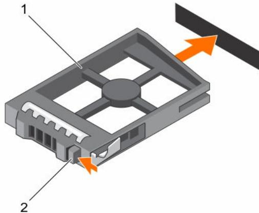
**Figure 22. Removing and installing a 2.5 inch hard-drive blank**
