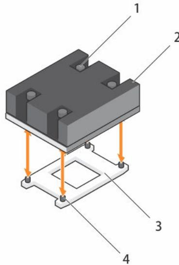
**Figure 39. Removing and installing a processor heat sink**
