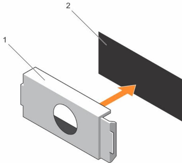
**Figure 43. Removing and installing the power supply blank**
