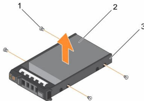
**Figure 26. Removing and installing a hard drive into a hard-drive carrier**
