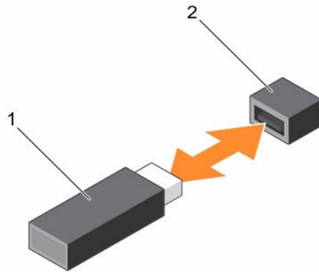
**Figure 31. Replacing the internal USB key**
