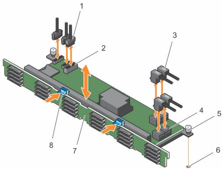
**Figure 52. Removing and installing the 1.8 Inch (x24) hard-drive backplane**
