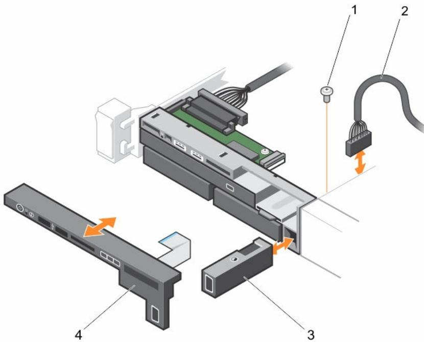
**Figure 57. Removing and Installing the VGA Module**
