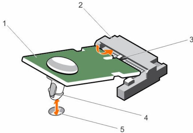
**Figure 59. Installing the TPM**
