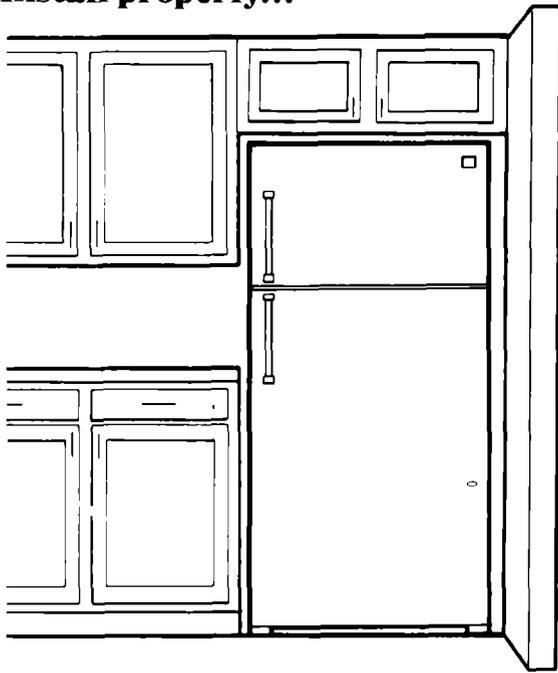
1. Allow 3 inches (7.5 cm) between overhead cabinets and the refrigerator top.
