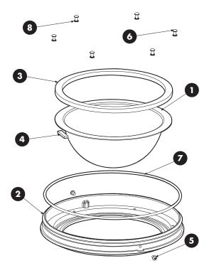
Figure 4. Exploded Assembly Diagram-Lower Dome, Pendant Models
