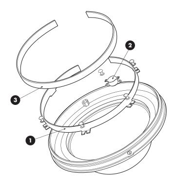
Figure 6. Exploded Assembly Diagram-Heater Segment in Lower Dome
