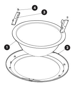
Figure 3. Exploded Assembly Diagram-Lower Dome, In-Ceiling Models
