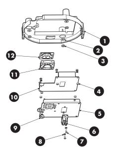
Figure 2. Exploded Assembly Diagram-Back Box Electronic Assembly
