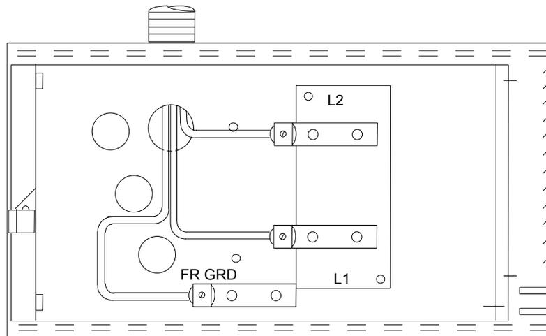
**Figure 5 - Power shelf individual AC connection**
