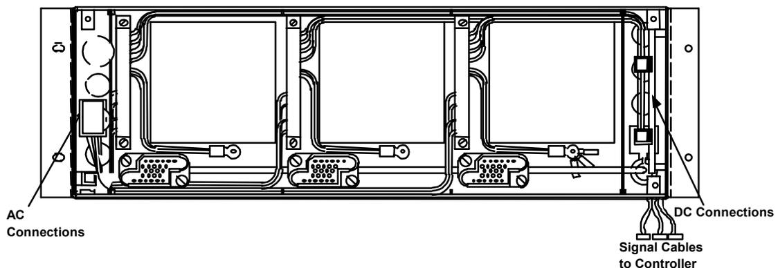
**Figure 2 - MPS75 Modular Power shelf- NT5C10C with 26-pin signal connectors**
