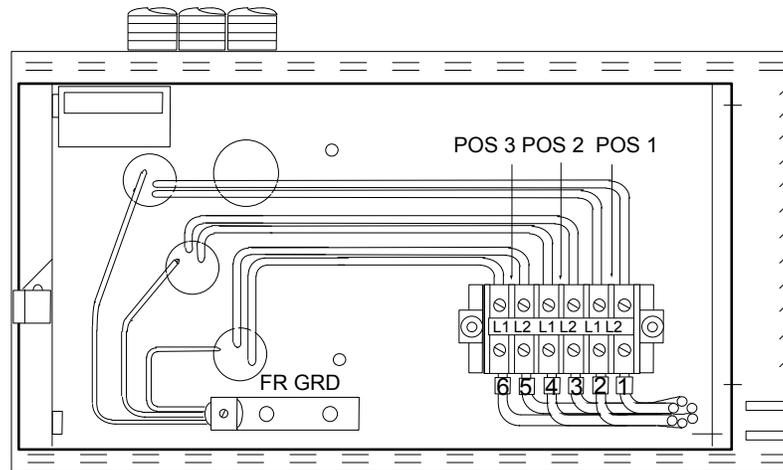
When cabling the AC to the power shelf, make sure that each corresponding safety ground wire is properly connected to the terminal designated FR GND.
