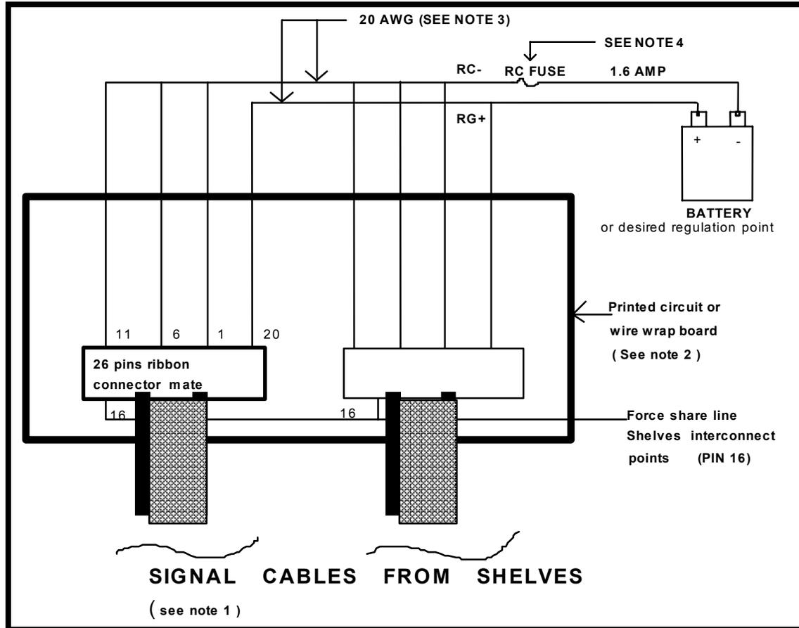
**Note 1:** Refer to MS5C06 for available signal cables of different lengths, to connect from the shelf backplane rectifier position to the remote sensing point.
