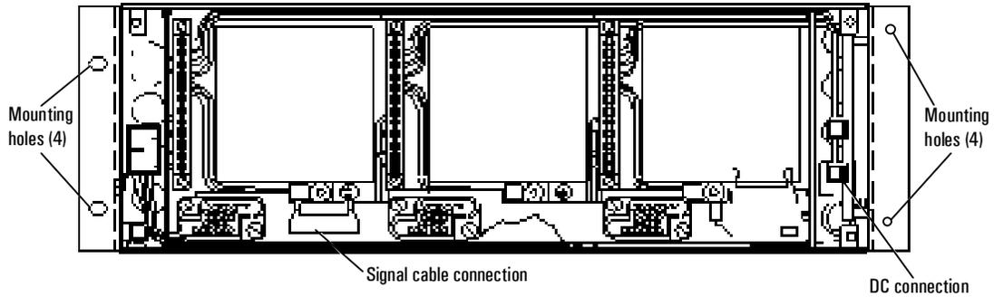
**Figure 3 - NT5C06D Switch Mode Rectifier**
