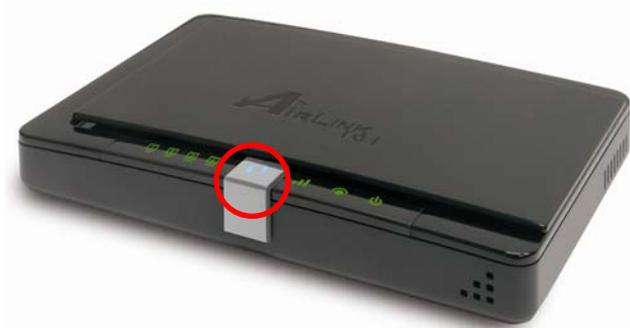
**Step 3** The Router will now start the handshake with the wireless adapter. When you see the window below, the wireless connection has been established.
