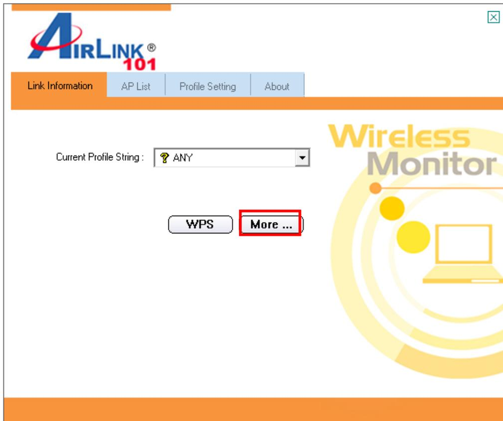
**Step 9** Verify that you are receiving adequate Signal Strength and Link Quality and that you have been assigned a valid IP address (instead of all 0's).
