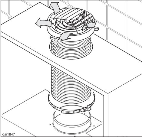
If site conditions are not suitable for the hood to be used for air extraction, the appliance must be converted for recirculation using the following installation kit. It can be ordered from your Miele dealer or the Technical Service Dept.
