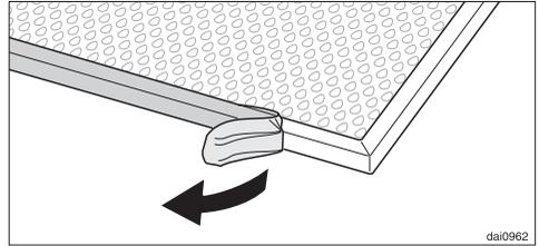
Before using the appliance remove the grease filters and remove the protective foil from the filter frame. Insert the grease filters back into place.
