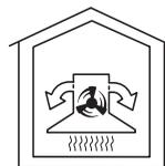
Air is drawn through the grease filters and **active charcoal filters**. The filtered air is then recirculated back into the kitchen through a grille at the top of the hood's chimney.
