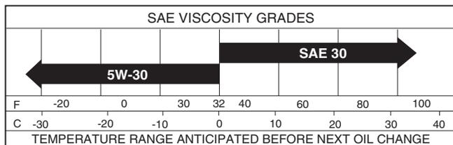
**NOTE:** Although multi-viscosity oils (5W30, 10W30 etc.) improve starting in cold weather, they will result in increased oil consumption when used above 32°F. Check your engine oil level more frequently to avoid possible engine damage from running low on oil.
