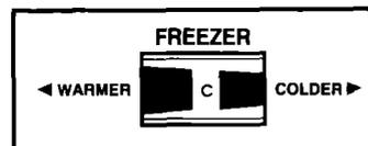
The settings indicated above should be correct for normal, household refrigerator usage. The controls are set correctly when milk or juice is as cold as you like and when ice cream is firm. If you need to adjust these settings, see "Changing the control settings" on page 8.
