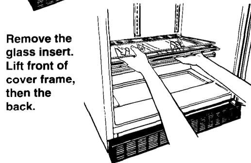
Remove the glass insert. Lift front of cover frame, then the back.
