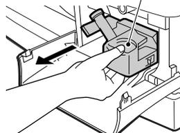
**3** Remove the new drum cartridge from the protective bag and remove the protective cover from the cartridge. Gently install the new drum cartridge.
