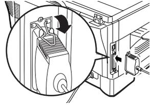
**3** Insert the other end of the cable into the interface connector of your computer.
