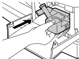
**4** Gently install the TD cartridge. To install the TD cartridge, see "TD CARTRIDGE REPLACEMENT" (p.84)
