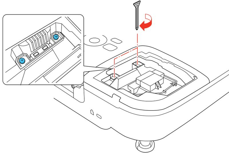
9. Replace the lamp cover and tighten the screw to secure it.
