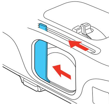
2. To cover the lens or temporarily turn off the projected picture and sound, slide the **A/V Mute** slide cover closed.
