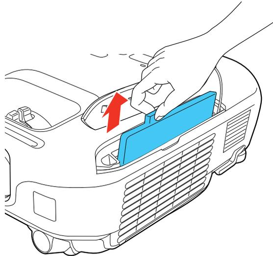
**Note:** Air filters contain ABS resin and polyurethane foam. Dispose of used air filters according to local regulations.
