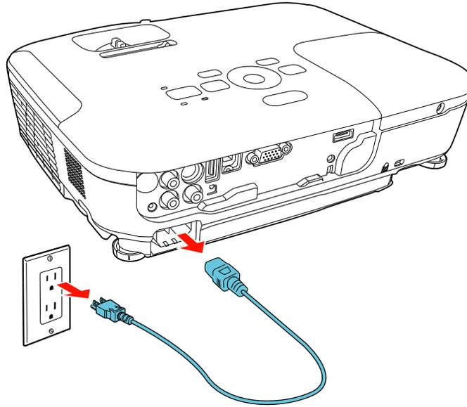
**Caution:** To avoid damaging the projector or lamp, never unplug the power cord when the power light is green or flashing orange.
