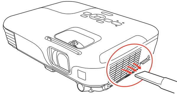
**Note:** You can remove the air filter so you can clean both sides of it. Do not rinse the air filter in water, or use any detergent or solvent to clean it.
