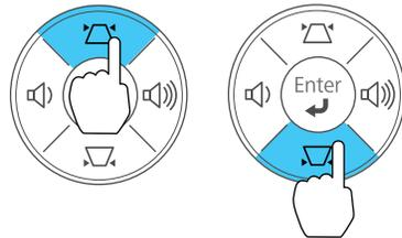
3. Press a keystone button on the projector's control panel to adjust the image shape.
