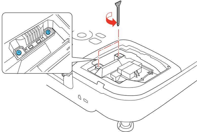
6. Lift up the lamp handle and gently pull the lamp out of the projector.
