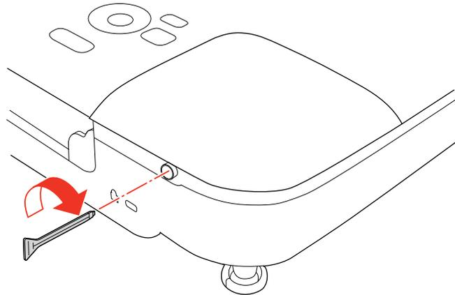
**Note:** Be sure the lamp cover is securely installed or the lamp will not come on.
