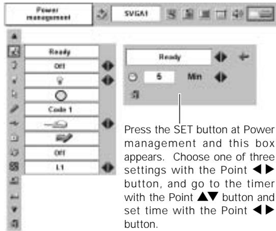
Press the SET button at Power management and this box appears. Choose one of three settings with the Point ◀▶ button, and go to the timer with the Point ▲▼ button and set time with the Point ◀▶ button.
