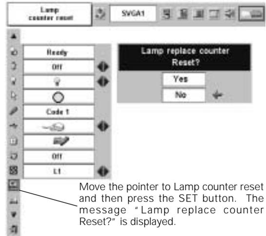
Move the pointer to Lamp counter reset and then press the SET button. The message "Lamp replace counter Reset?" is displayed.
