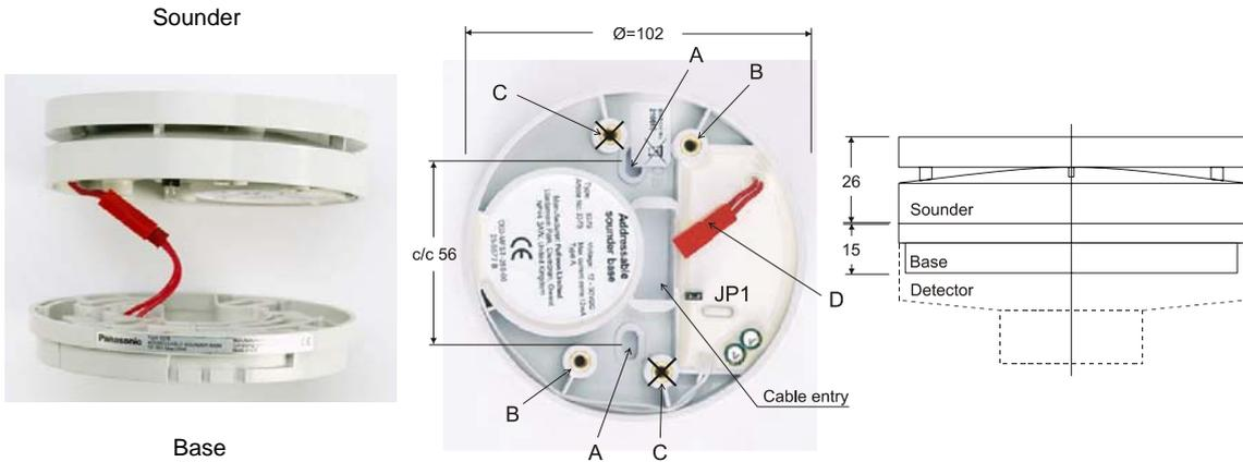
The sounder: **A** = Mounting hole (5 x 9.5) for the sounder. Between the sounder and the ceiling can an 8 mm spacer ( $\varnothing_o = 13$ ) be mounted for easier access of surface mounted cables. **B** = Mounting hole (M4) for the base. **C** = Must not be used. **D** = Connector for the base connector. **JP1** = Jumper (in position = high output; removed = low output). Analog detector types 33xx and 430x can be plugged in the base.
