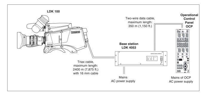
In this mode the camera is connected to a base station via a Triax adapter and cable. Remote control of the camera is achieved by a remote control panel of the Series 9000 Control System. This can be an
