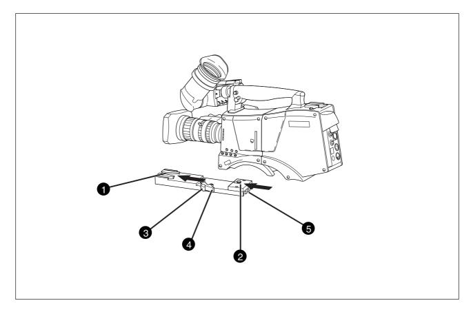
To mount the camera on a tripod, the tripod plate (LDK 5030/00 is delivered as standard) must first be attached to the tripod.
