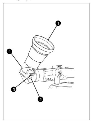
If you regularly use the viewfinder at a distance, for example, when you use the camera in the hand-held position, it is recommended that you fit the optionally available wide angle eyepiece (LDK 5390/00).
