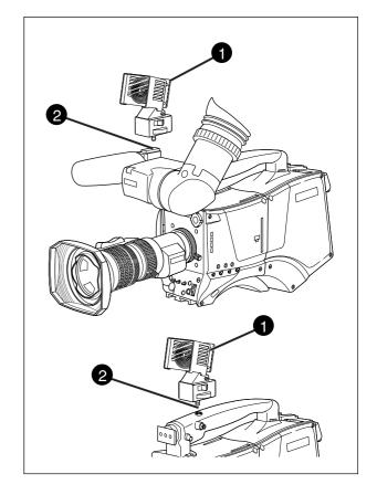
To mount a top light  $\ensuremath{\bullet}$  onto the camera, proceed as follows:
