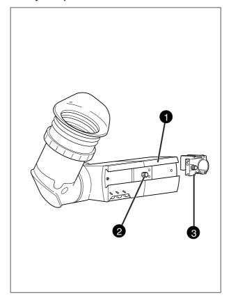
A left eye adapter is optionally available (LDK 5390/10) to allow the viewfinder to be used with the left eye.
