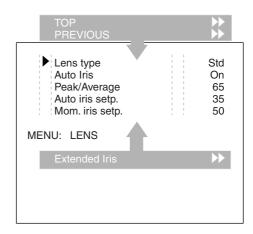
The LENS menu above shows the items displayed when you first enter the menu and the other items that are available by scrolling up or down with the Rotary control.
