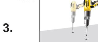
Drill 4 pilot Holes with an electric drill & 1/16" bit. Make sure that nothing is behind the mounting surface that can be damaged when drilling the holes. (Figure 4)
