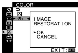
The picture disappears while the color is being restored (about 2 seconds). After the color is restored, the picture reappears on the screen again.
