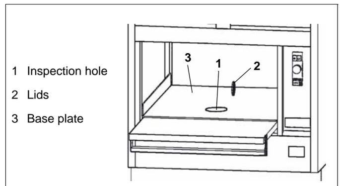
Fig. 12 Checking the pilot flame
