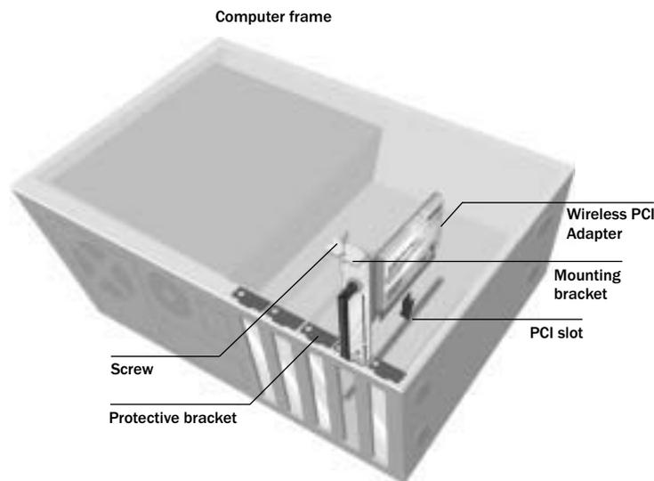
6. Screw the bracket of the wireless PCI adapter securely to your computer's frame.
